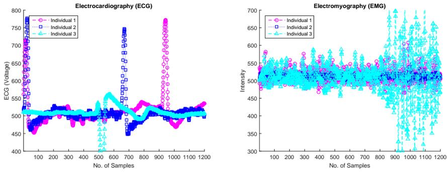
**Fig. 3.** ECG (on the left) and EMG (on the right) samples obtained from BITalino.
