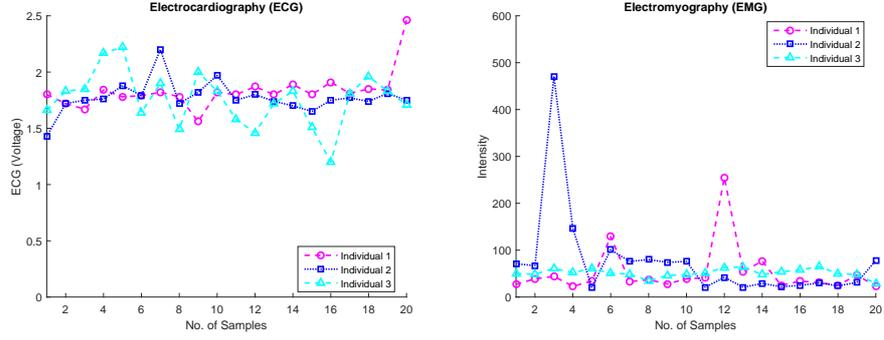
**Fig. 2.** ECG (on the left) and EMG (on the right) samples obtained from Arduino.
