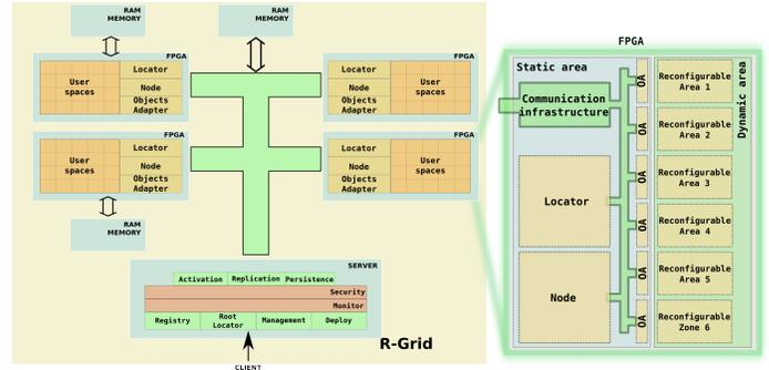
Figure 3. R-GRID Physical Architecture
