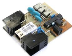
Fig. 3. Our L-EMD prototype: ethernet interface, PIC16F876A microcontroller and three triacs for power control switching.
