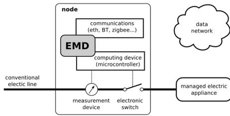
Fig. 1. Block diagram of the general EMD structure.
