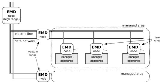
Fig. 2. Example of deployment where different types of EMD are used.
