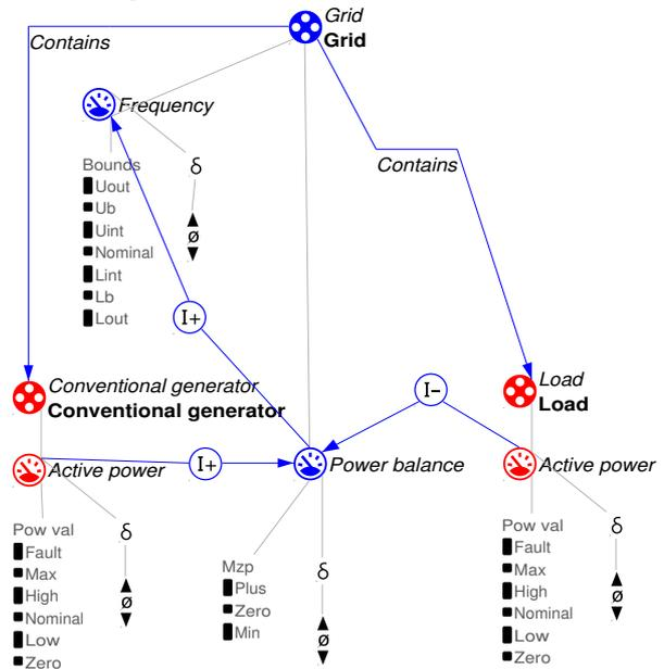
Fig. 4. Frequency deviation model fragment.
