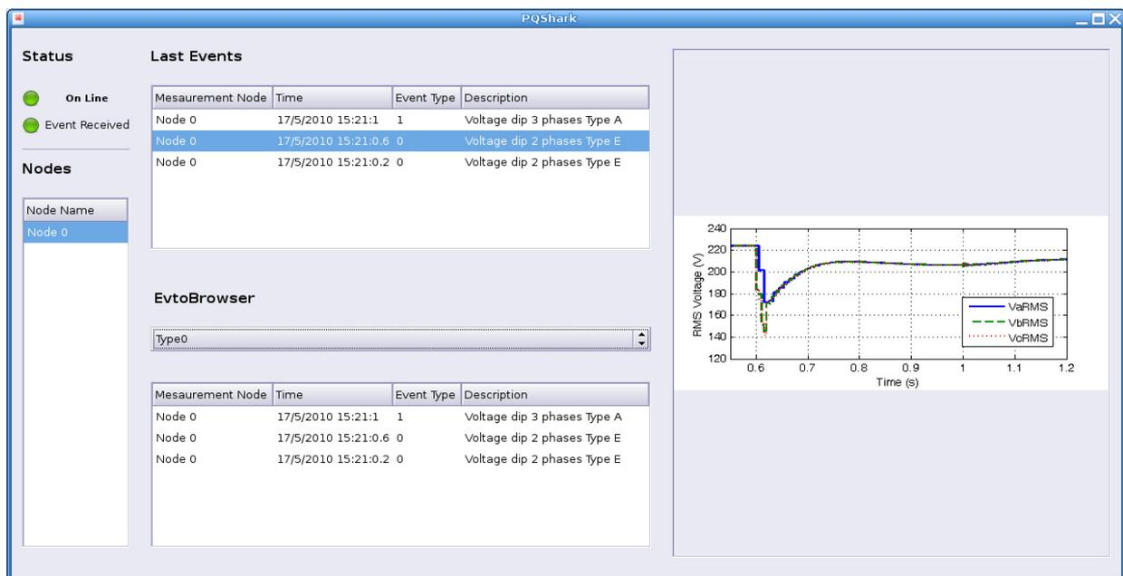
Fig. 11. Screen-shot of the monitoring System.
