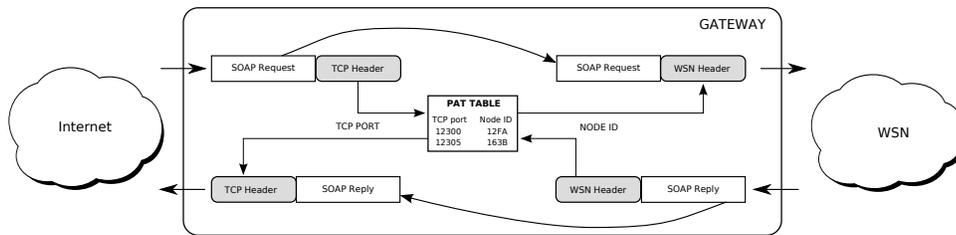
**Fig. 4.** Simplified gateway process
