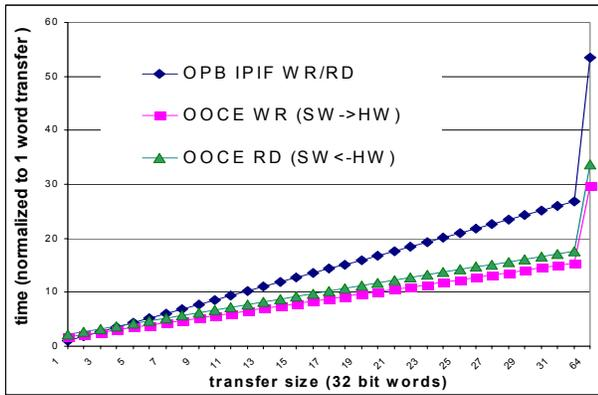
Figure 6. Performance of on-chip read/write transactions using Xilinx IPIF and OOCE.
