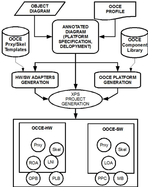
Figure 1. Interface synthesis and prototype platform generation flow in OOCE.
