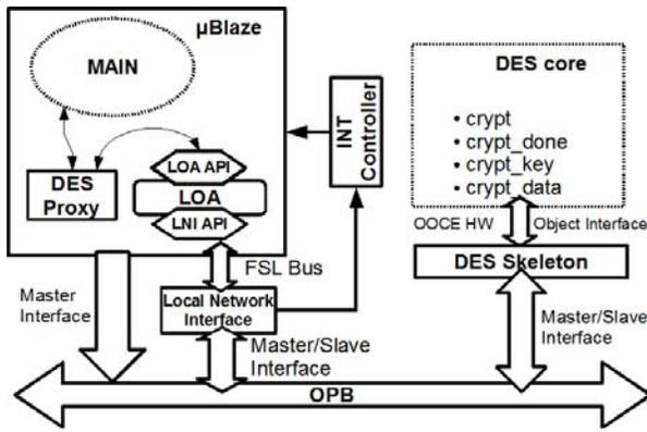
Figure 3. Derived HW and SW platform.
