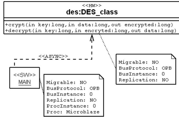
Figure 2. UML OOCE annotated diagram for a minimal cryptographic application.
