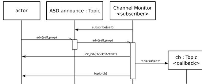
**Fig. 1.** Sequence diagram for Channel Monitor Service.
