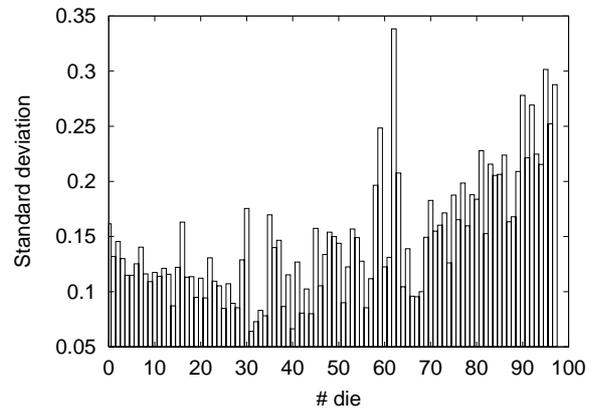
Figure 4: **Standard deviation of current differences of every die and a golden circuit. The x-axis is the same than fig. 3.**
